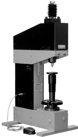
Figure 3-1. Brinell tester. (Reproduced by permission of Newage Testing Instruments, Inc., Southampton, PA, http://www.hardnesstesters.com/brinell-hardness-tester.htm .)
