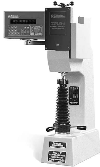
Figure 3-2. Rockwell tester. (Reproduced by permission of Newage Testing Instruments, Inc., Southampton, PA, http://www.hardnesstesters.com/rockwell-hardness-tester.com .)
