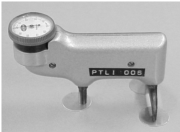
Figure 3-3. Barcol tester. (Reproduced by permission of Plastics Technology Laboratories, Inc., Pittsfield, MA, http://www.ptli.com .)
